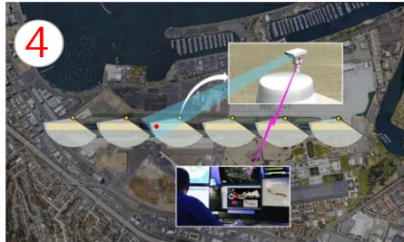
4 Radar unit detects FOD within 2 minutes, coordinates relayed to camera system and identifies FOD object.
